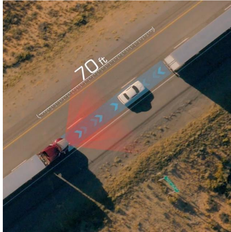
If driver does not respond, system radar detects cut-in vehicle and automatically begins to back off follow truck
